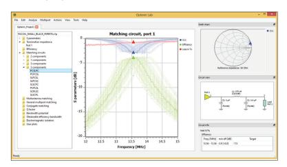
Tolerance analysis is an important part of the total NFC performance analysis. Optenni Lab enables tolerance analysis being carried out directly on the vendor library components.
